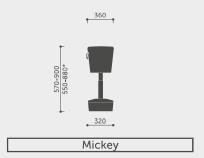
$<sup>\</sup>boldsymbol{\ast}$  Seat height is measured according to PN EN 16139 norm (with seat burden).
